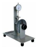
This mechanism demonstrates relative motion between a rotating eccentric mamber (cam) in degrees and a sliding member (follower) translation in millimeters such as found in internal combustion engine
