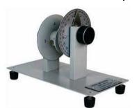
This mechanism demonstrates relative angular motion in degrees between two shafts with parallel but displaced axes
