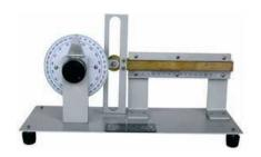
This mechanism demonstrates relative motion between a crank rotation in degrees and a yoke translation in millimeters
