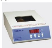
S.S block chamber can act as water bath
